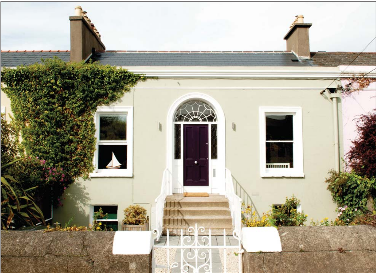
(above) Preserving the historic front facade was essential as the house sits in the middle of a Victorian terrace, and the new double-glazed sash windows replicate the historical look; (opposite) a void above the new kitchen brings plenty of light into the building
